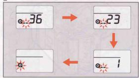
2. When the film is fully rewound, only [ **Q** ] blinks on the LCD panel.
