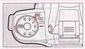
In the multi(6)-segment metering mode, the metering system automatically measures light in six different zones, enabling proper exposure value in a wide variety of normal and adverse lighting conditions, such as a backlit condition.
