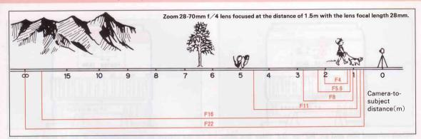
Depth of field refers to the range around the optimum focusing point of the subject in which the elements at different distances are in focus. The depth of field increases as the aperture is closed down, the focal length of the lens becomes shorter, or the subject is positioned farther away.
