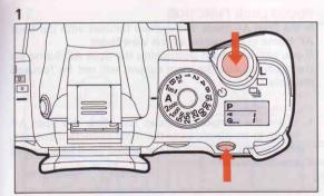
Select the Spot AF Mode to critically focus on a specific spot of the subject which is in the spot AF autofocus frame.
