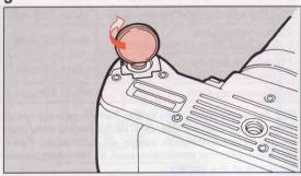
3. Turn the battery chamber cover screw in the direction of the arrow to lock it securely.
