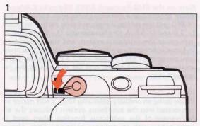
You can switch between the panoramic format and standard format picture taking mode in the middle of the roll by moving the panorama lever. The panoramic format picture allows horizontally positioned dynamic pictures to be taken (the panoramic format is approximately 13x36mm on the film).
