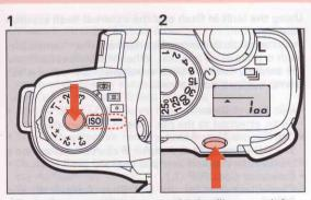
This camera automatically reads the film speed from the film's DX code. However, the film speed setting can be changed. If you use a non-DX coding film, set the film speed manually.
