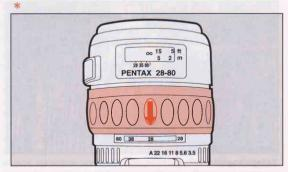
Using the manual zoom function with an FA zoom lens attached
