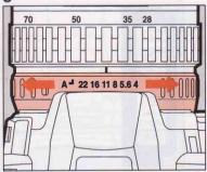
3. Adjust the desired aperture by the lens aperture ring.
