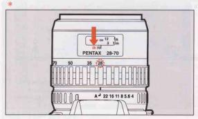
When infrared film and an "R2" or "O2" filter are used, the focal point is different from that of ordinary film exposed in visible light. The autofocus system cannot compensate for this difference automatically.
