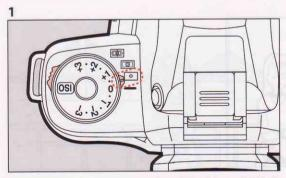
The desired metering mode, multi(6)-segment metering, spot or center weighted metering mode can be selected.
